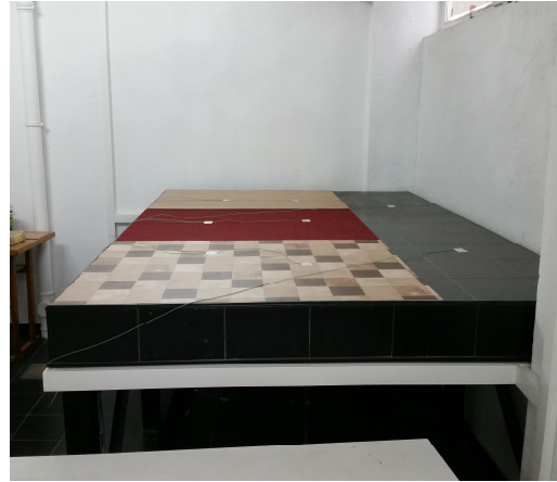
Fig. 6. TABS radiant surface in the faculty laboratory
