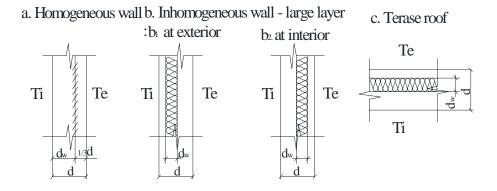
Fig. 1. Accumulation of moisture from condensation from different types of elements
