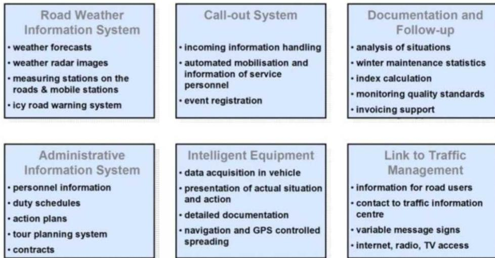
Fig. 1. Component of a Winter Maintenance Management System – WMMS [1]
