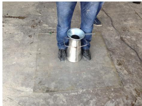
Fig. 3. *The cone spread equipment*
