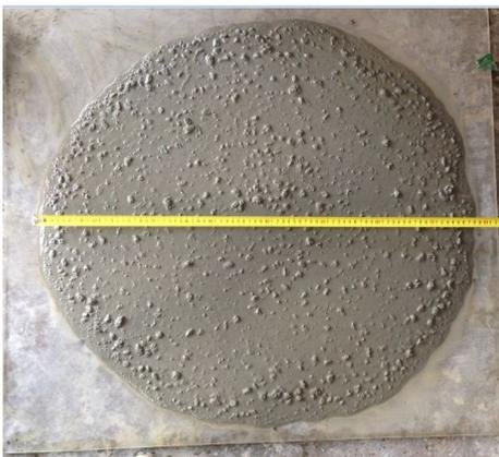
Fig. 7. Spread after preparation
