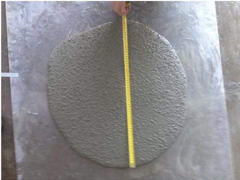
Fig. 4. *The Spread Test*
