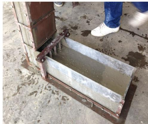
Fig. 8. L box after preparation
