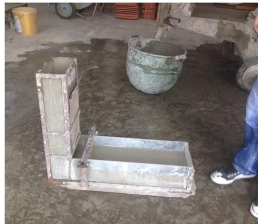
Fig. 6. *The L box test*
