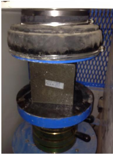
Fig. 11. *Compression Strength determination*
