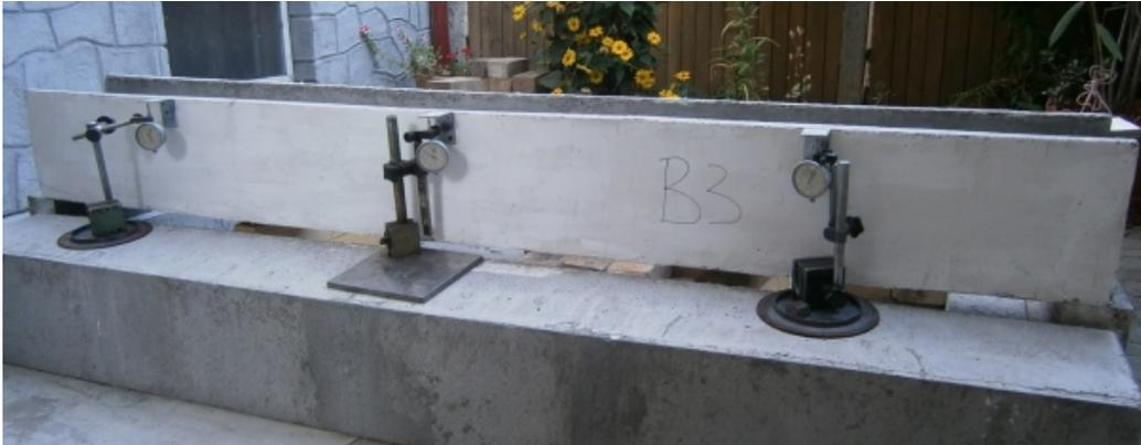
Fig. 1. *Lintel ready for testing*
