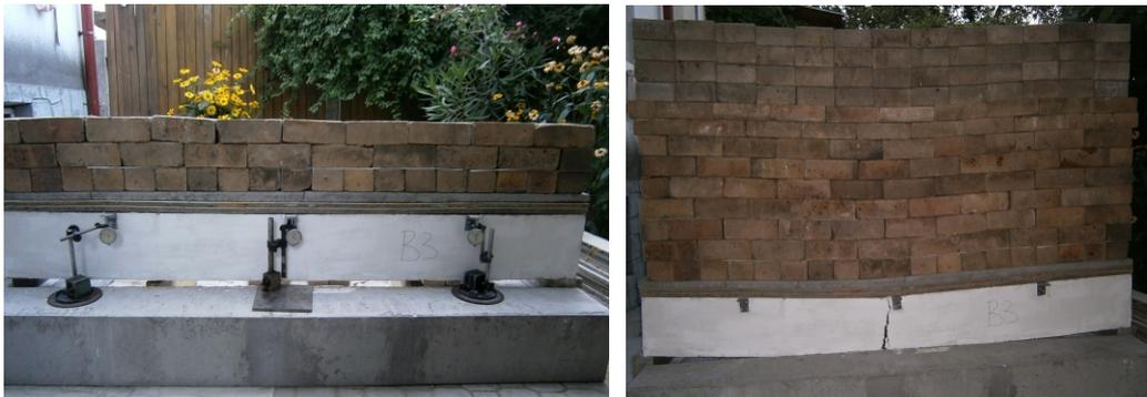
Fig. 2. *Lintel during test and failure moment*
