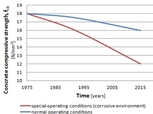
Fig. 8. Operating conditions influence in time over concrete compressive strength
