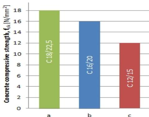
Fig. 6. Operating conditions influence over the concrete class:
