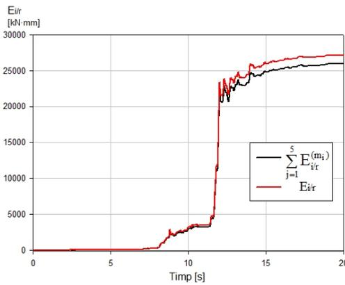
Fig. 7. Total seismic input energy five levels stiff frame. Focsani, 10%
