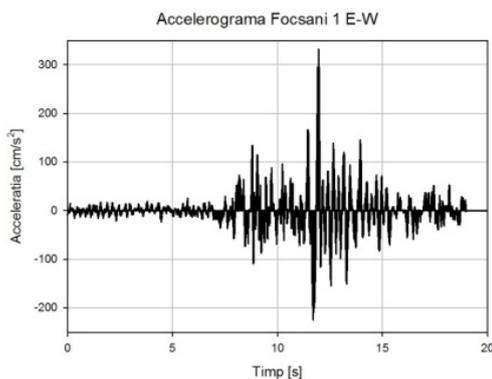
Fig. 2. Focsani 1986 accelerogram
