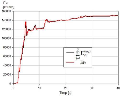
Fig. 9. Total seismic input energy five levels flexible frame. El Centro, 5%
