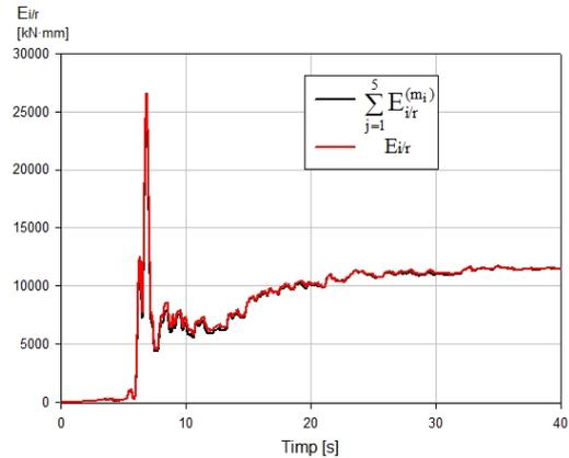
Fig. 3. Total seismic input energy. Five levels frame moderate stiff. Vrancea, 2%
