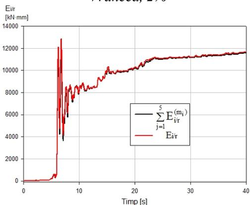
Fig. 5. Total seismic input energy five levels stiff frame. Vrancea, 5%
