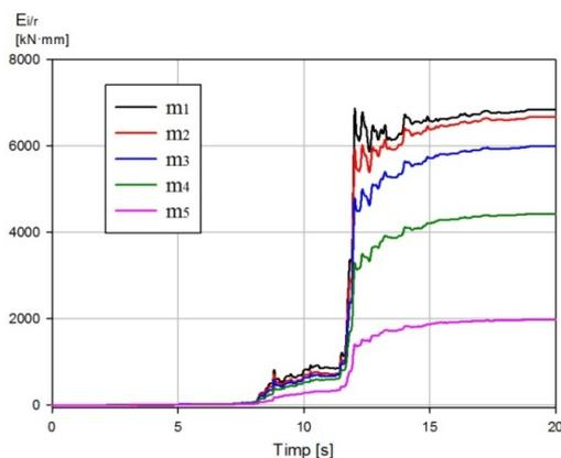
Fig. 8. Mass energy components five levels stiff frame. Focsani, 10%
