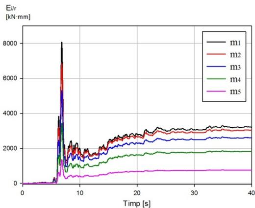
Fig. 4. Mass components of seismic input energy. Five levels stiff frame Vrancea, 2%
