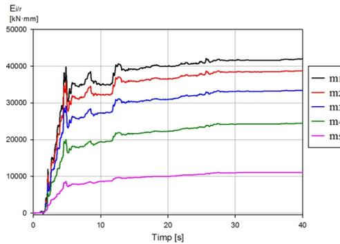
Fig. 10. Mass energy components five levels flexible frame. El Centro, 5%
