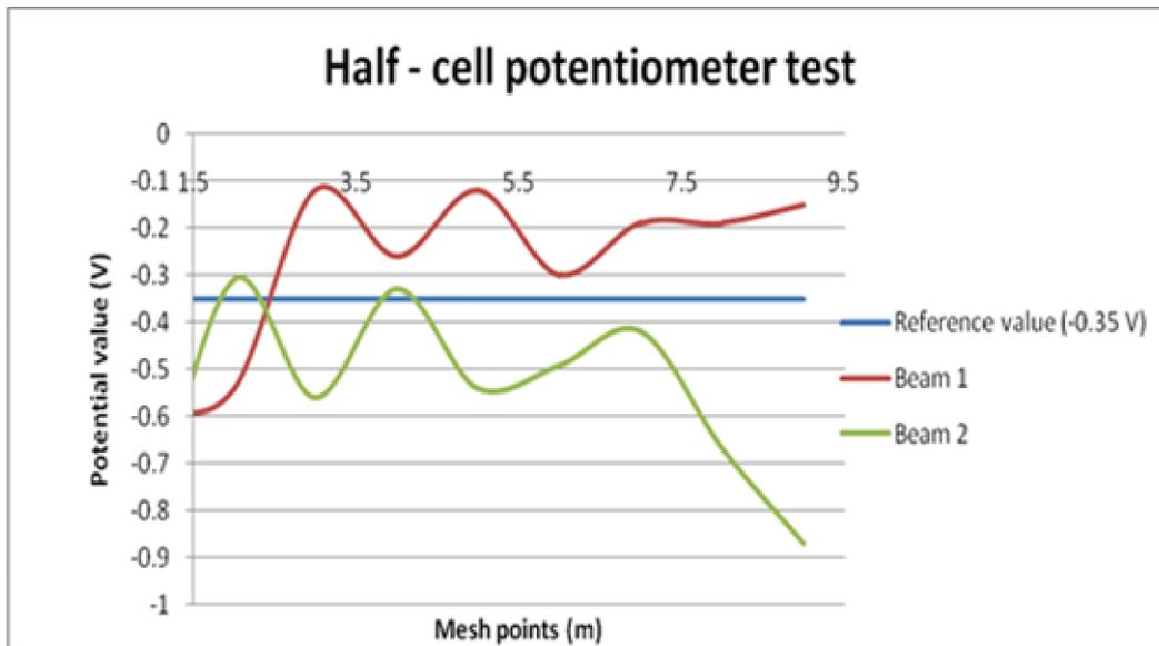
Fig. 4. Beams corrosion results
