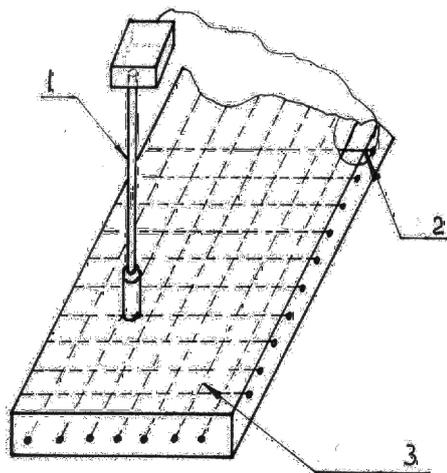
1. Half-cell potentiometer; 2. Reference re-bar; 3. Tested element
