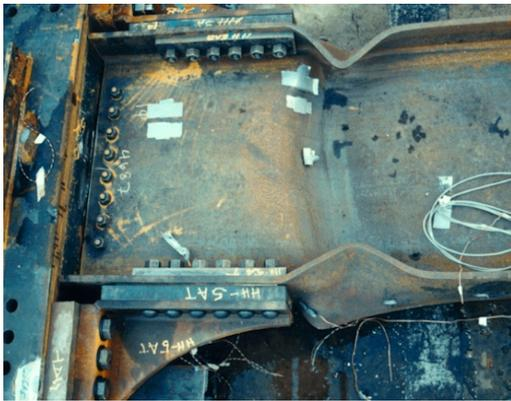
Fig. 5. Kaiser Bolted Bracket connection failure [6]
