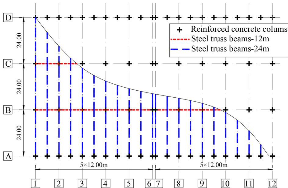
Fig. 1. *Structural elements arrangement*
