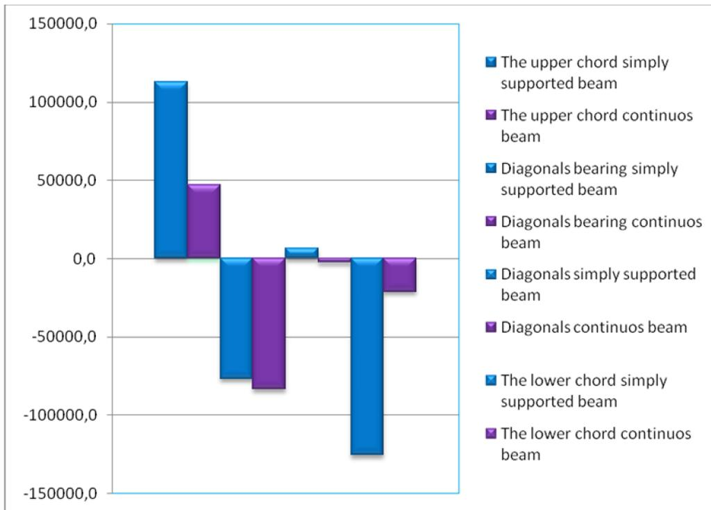
Fig. 8. *The graphic comparative representation of strains in trusses elements*
