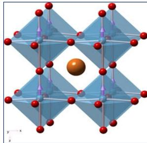
Fig. 1. Atomic structure - Barium Titanate
