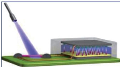
Fig. 17. *A ZnO based UV nanosensor coupled with a nanogenerator in an energetic independent nanosystem*
