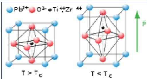
Fig. 2. Unit cell of Tetragonal Lead Titanate
