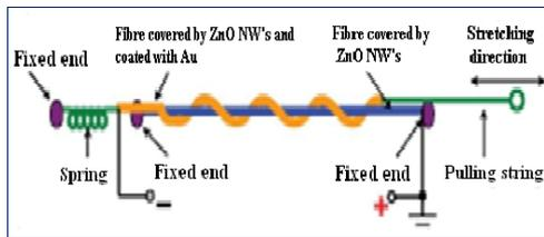
Fig. 16. *ZnO nanowires grown on textile fibers*
