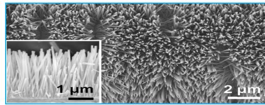
Fig. 12. Arrays of ZnO nanowires grown either on a GaN substrate or sapphire substrates that are covered by a thin layer of ZnO film, serving as a common electrode for directly connecting the nanowires with an external circuit.
