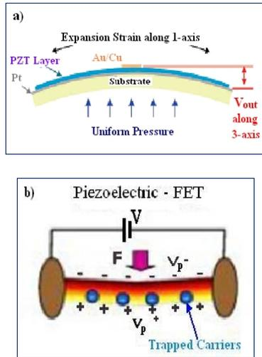
Fig. 10. a) A PZT layer having the substrate, the top and base electrodes indicated;
