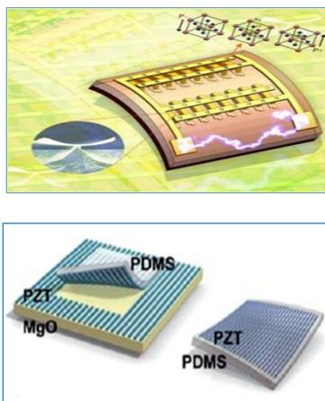
Fig 14. *Flexible nanogenerators thin film type, without moveable, quick wearable constitutive parts*[19]
