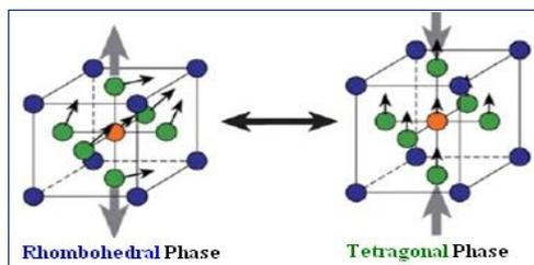
Fig. 5. Stress-induced phase transition in PZT. Blue = Pb atoms. Green = O atoms. Orange = either Ti or Zr atoms
