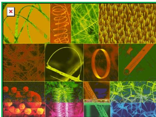
Fig. 9. ZnO nanostructures (nanocombs, nanorings, nanohelices/nanosprings, nanobows, nanobelts, nanowires, nanocages)
