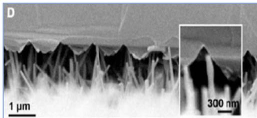
Fig. 11. The top zigzag electrode interacting with vertically aligned array of ZnO nanowires
