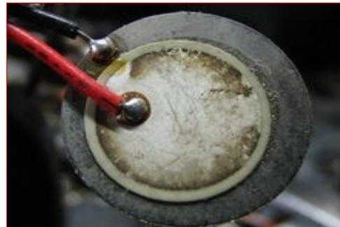
Fig. 6. Piezoelectric ceramic disc attached to a thin flexible metallic disc
