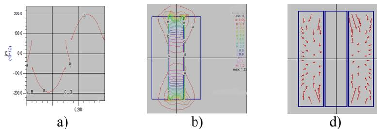
Fig. 4. Simulations for  $\mu_r = 10000$  and  $z_c = 128$  mm: a) molecular current density; b) Contour of  $B = ct.$ ; c) Magnetic force
