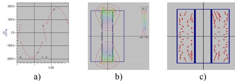
Fig. 3. Simulations for  $\mu_r = 1000$  and  $z_c = 128$  mm: a) molecular current density; b) Contour of  $B = ct.$ ; c) Magnetic force
