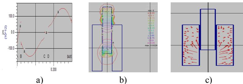
Fig. 2. Simulations for  $\mu_r = 10000$  and  $z_c = 113$  mm: a) molecular current density; b) Contour of  $B = ct.$ ; c) Magnetic force
