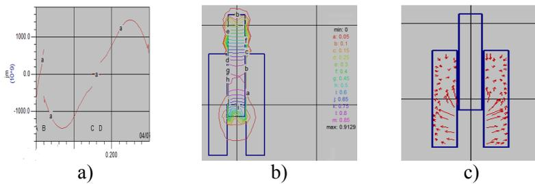
Fig. 1. Simulations for  $\mu_r = 1000$  and  $z_c = 113$  mm: a) molecular current density; b) Contour of  $B = ct.$ ; c) Magnetic force
