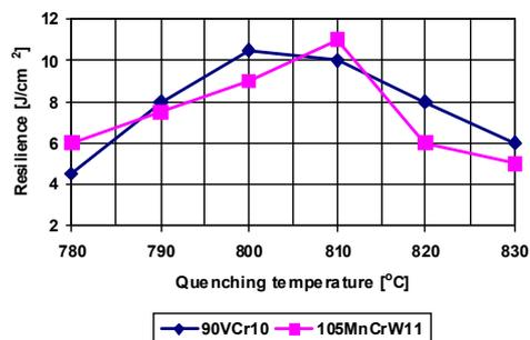
Fig. 7. Quenching temperature influence on the specific impact energy
