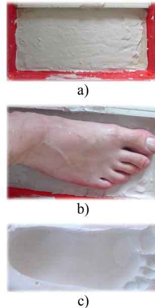
Fig. 4. Stage of molds: a) casting and levelling the plaster layer; b) fingerprinting; c) mold obtaining
