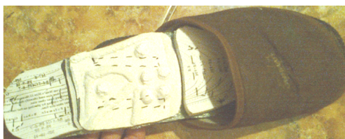
Fig. 2. Example of the arrangement of samples on sanitary silicone insoles on the shape memory textile insoles
