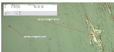
Fig. 15. Digital image for wood lens scratches (500x)
