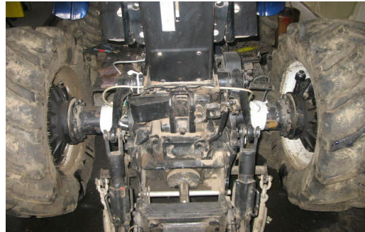
Fig. 6. Complete assembly of sensors on the back axle of the tractor
