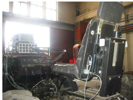
Fig. 7. Two accelerometers mounted to the tractor seat
