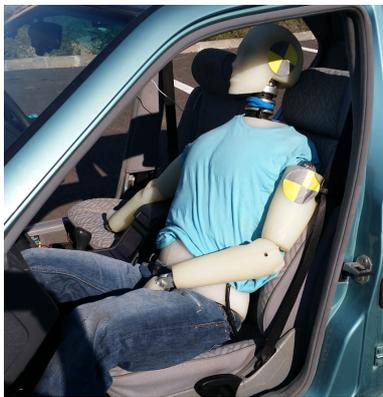
Fig. 17. Custom built crash test dummy
