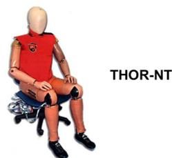
Fig. 16. *THOR test dummy*
