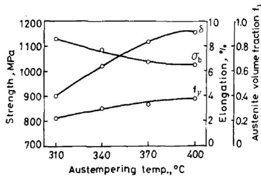
Fig. 3. Effect of austempering temperature on microstructure and mechanical properties [13]
