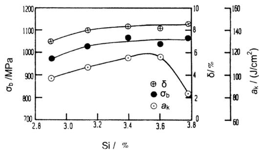
Fig. 4. Effect of Si on mechanical properties of ADI weld [14]
