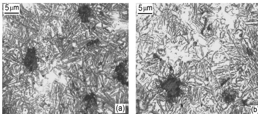
Fig. 1. Microstructures of austempered specimens at 375 °C for 20 min (a) and 100 min (b). Light regions are austenite [2]
