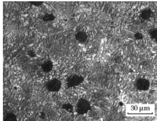
Fig. 2. *Microstructure of base material (ADI) consisting of acicular ferrite, retained austenite and nodular graphite [3]*
