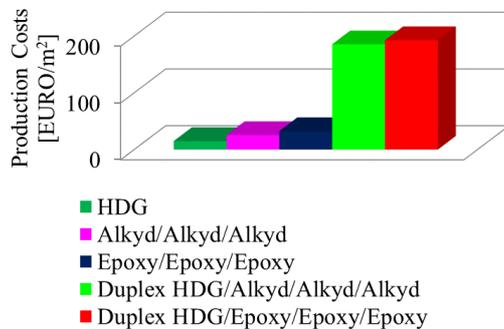
Fig. 2. Production costs of corrosion protection
