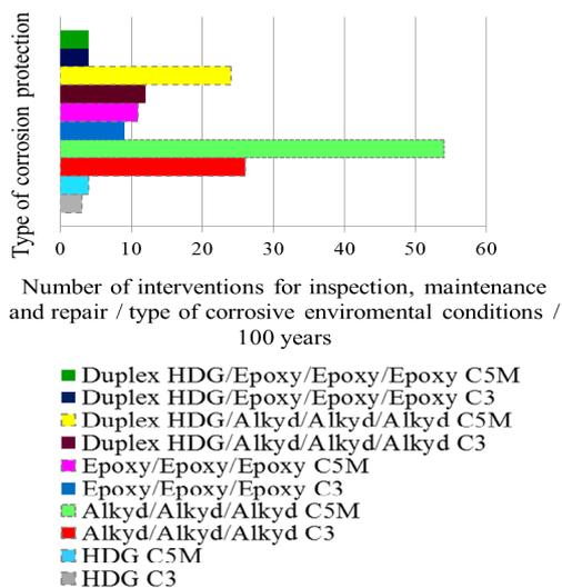
Fig. 6. Number of maintenance interventions required, depending on the corrosiveness of the environment, on the designed lifetime (100 years)
