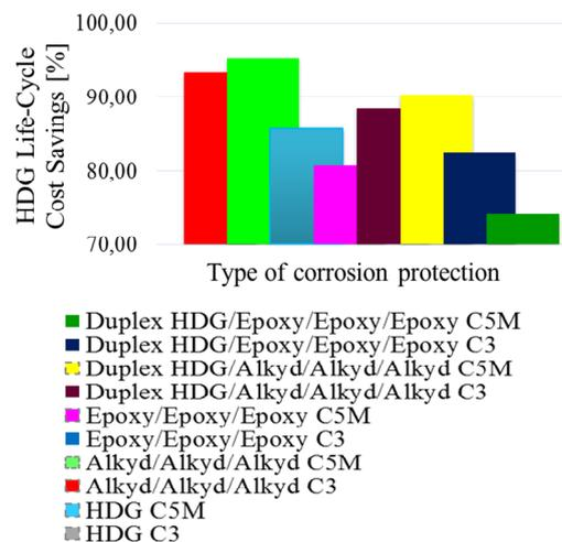
Fig. 7. Reducing costs during the lifetime of the considered systems when using corrosion protection by galvanizing HDG
