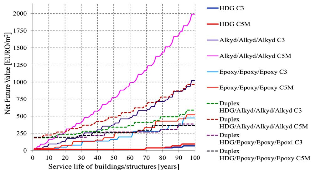
Fig. 3. Evolution of corrosion protection costs over the entire lifetime
