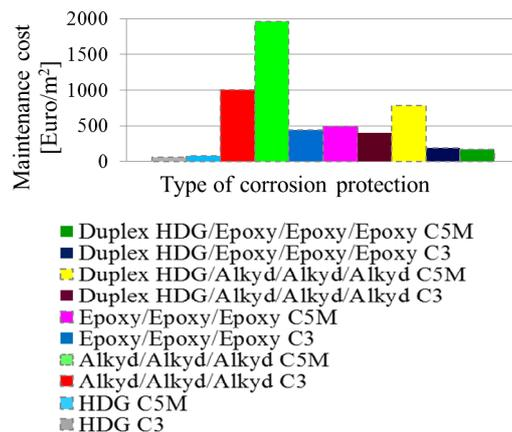
Fig. 5. Costs of maintenance and repair of corrosion protection, depending on the corrosiveness of the environment, on the designed lifetime
