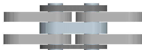
Fig. 2. I.T. chain construction top view
