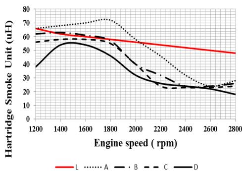
Fig. 4. *Smoke emission versus speed at full load*
