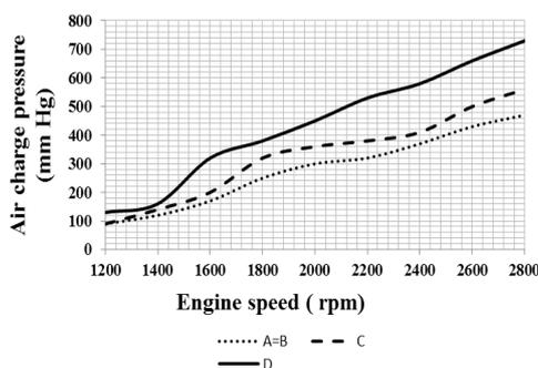
Fig. 5. *Air charge pressure versus speed*
