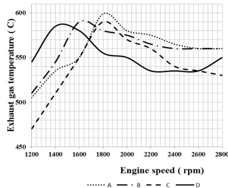
Fig. 6. *Exhaust temperature versus speed*
