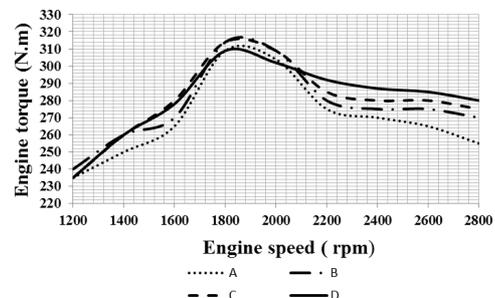
Fig. 2. Torque versus speed at full load
