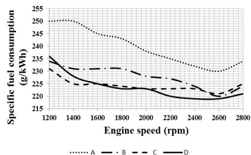
Fig. 3. Specific fuel consumption versus speed at full load
