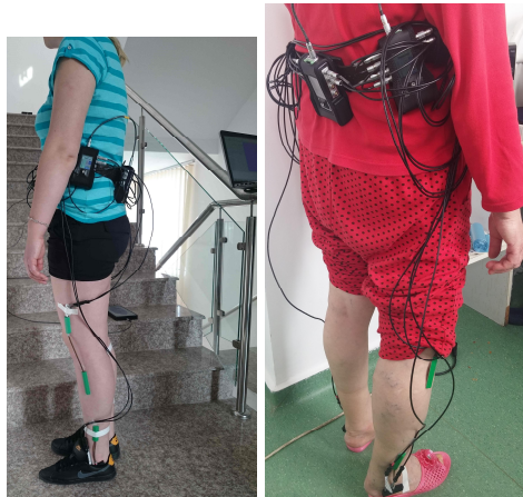
Fig. 3. Fixation of the electro-goniometers on the lower limbs.
