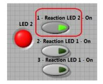
Fig. 4. Example of virtual switch to validate the perception of light stimulus
