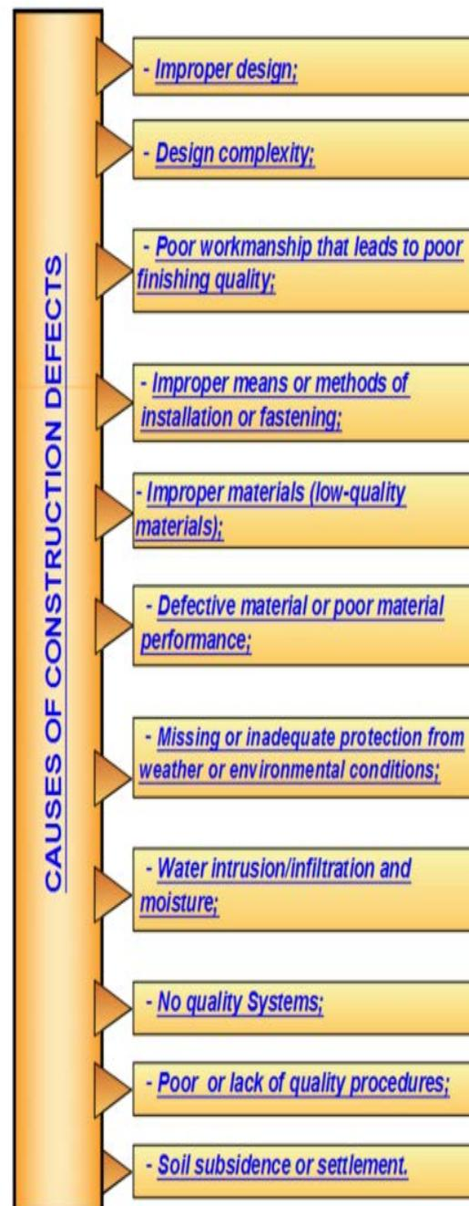
Fig. 1. Causes of construction defects
