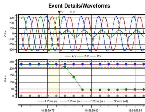
Fig. 3. Waveform of a mild bipolar negative transient
