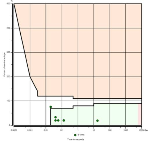
Fig. 2. The ITIC curve of the survey
