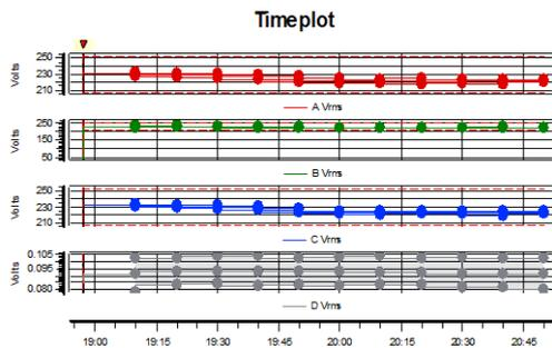
Fig. 1. Timeplot survey of the secondary voltage of the transformer substation
