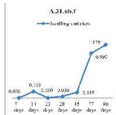
Fig. 4. Swelling values in time for asphalt base designed for light traffic A.31.nb.f
