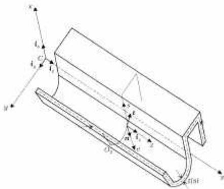
Fig. 1. Arbitrary open cross section
