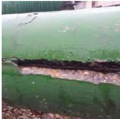
Fig. 2. Longitudinal crack after collapse
