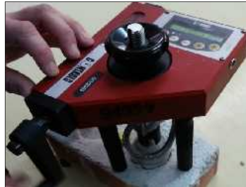
Fig. 4. a) Tensile strength testing device and b) Adherence testing device
