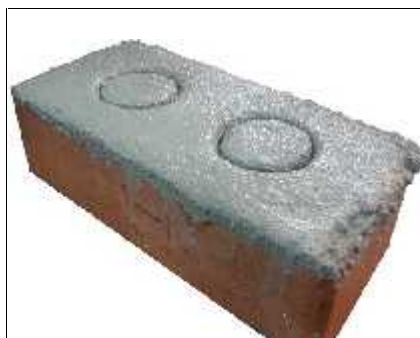
Fig. 5. The brick after plastering
