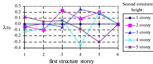
Fig. 6.  $\lambda_{Dc}$  values at each storey of the 6 storey structure at impact with buildings of 1 to 5 storey
