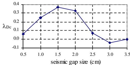
Fig. 8.  $\lambda_{Dc}$  values at 4 storey level as function of seismic gap size
