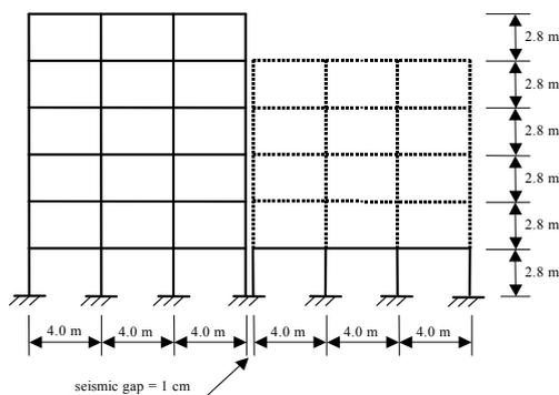
Fig. 2. Structures with different heights
