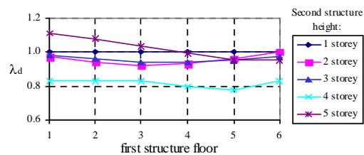
Fig. 5.  $\lambda_d$  values at each floor of the 6 storey structure at impact with buildings of 1 to 5 storey
