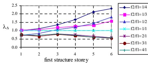
Fig. 4.  $\lambda_D$  values as function of natural frequencies of two adjacent buildings subjected to impact
