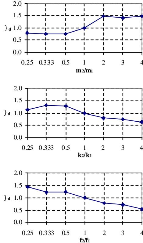
Fig. 3.  $\lambda_d$  values as function of the structural different characteristics of 2 adjacent buildings subjected to impact
