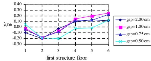
Fig. 7.  $\lambda_{Db}$  values at each storey of the 6 storey structure as function of seismic gap size
