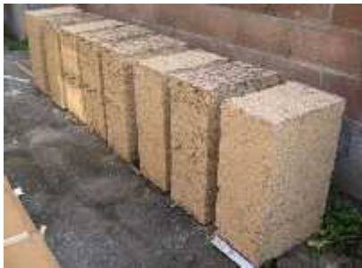
Fig. 9. Hemp-lime bricks can be used to build solid walls
