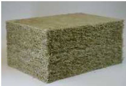
Fig. 7. Hemp-lime products (insulation).
