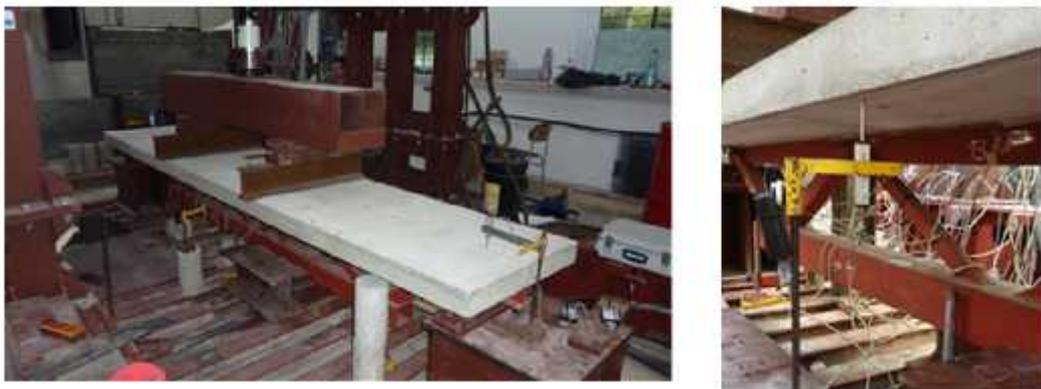
Fig. 6. Loading and measurement system
