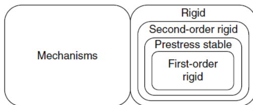
Fig. 4. Classification of frameworks with respect to rigidity properties [2]
