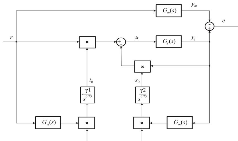
Fig. 4. Block diagram for a MRAC with a fractional-order adjustment rule
