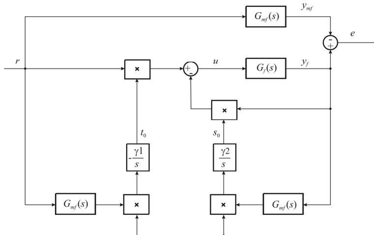
Fig. 7. Block diagram for a MRAC with a fractional-order reference model
