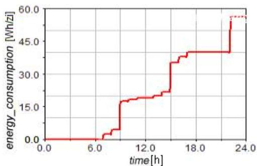
Fig. 5. The energy consumption for performing the step-by-step tracking
