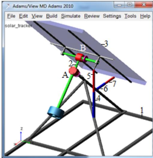
Fig. 1. Dual-axis equatorial tracker
