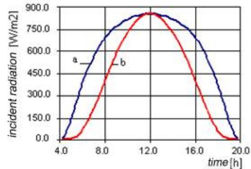
Fig. 4. The incident radiation with (a) / without (b) tracking
