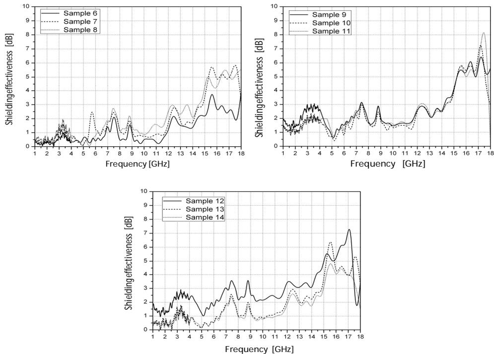
Fig. 3. *Shielding effectiveness versus frequency in domain 1-18 GHz for fibers with carbon insertion*
