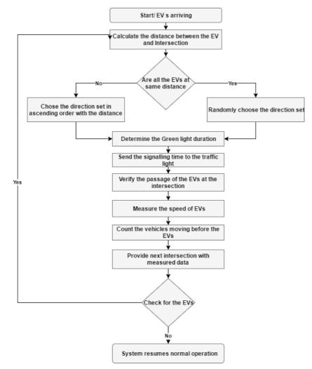
Fig. 3. Distance-based emergency vehicle dispatching algorithm
