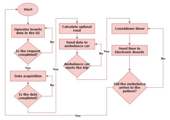
Fig. 4. Flowchart of Software application
