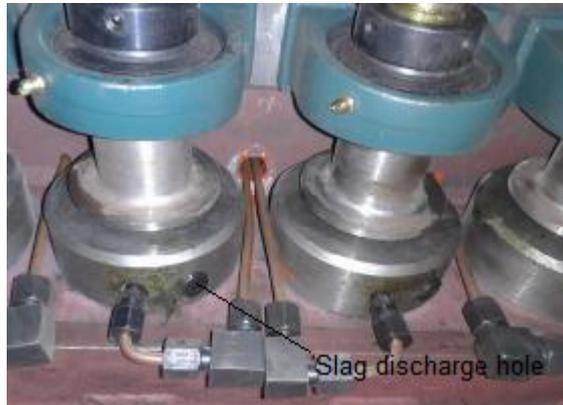
Fig. 5. Schematic diagram of slag discharge hole
