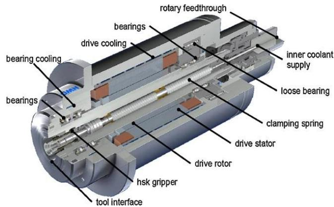
Fig. 1. Sectional view of a motorized spindle [courtesy: GMN]
