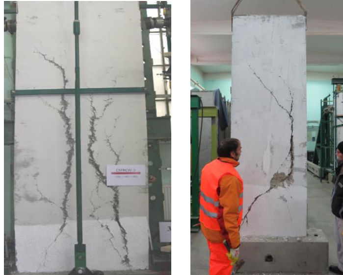
Fig. 3. Encountered type of failure - CSFRCW group of specimens - shear failure
