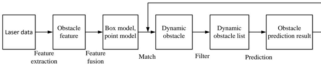
Fig.2 Dynamic obstacle detection tracking flowchart
