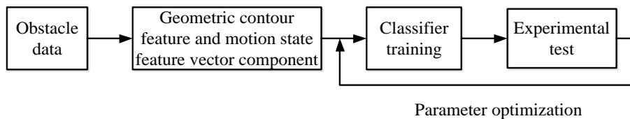
Fig.5 Flow chart of lidar identification method
