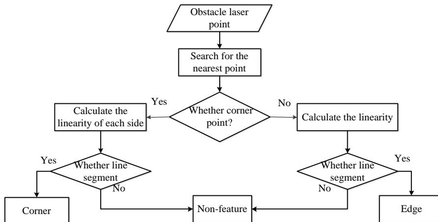
Fig.3 Flow chart of feature extraction algorithm
