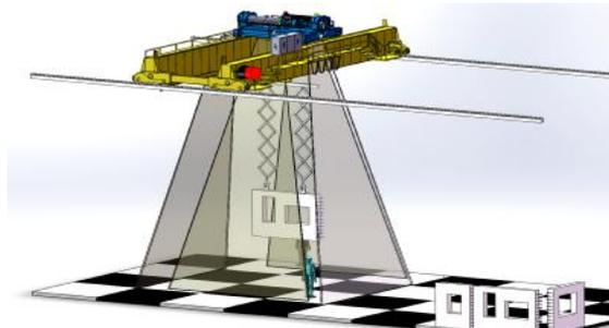
Fig.1 *Obstacle detection effect diagram during the process of transportation*
