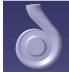
Fig. 2. 3D model of volute water body
