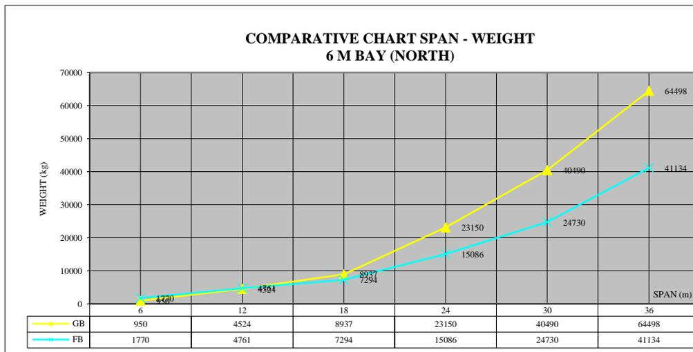
Fig. 3. Comparative chart span - weight. 6 m bay
