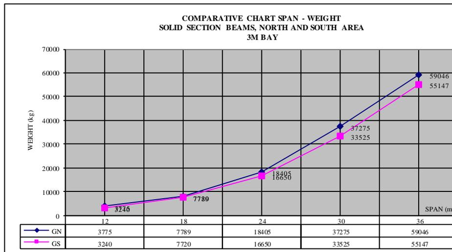
Fig. 5. Comparative chart span - weight, solid section beams, north and south area. 3 m bay
