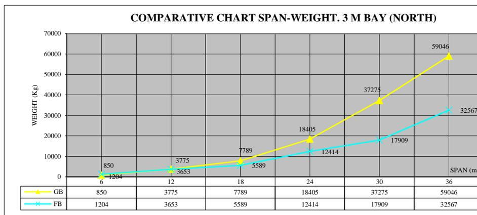
Fig. 1. Comparative chart span - weight. 3 m bay
