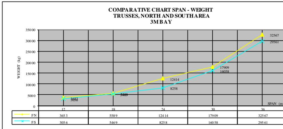
Fig. 6. Comparative chart span - weight, trusses, north and south area. 3 m bay
