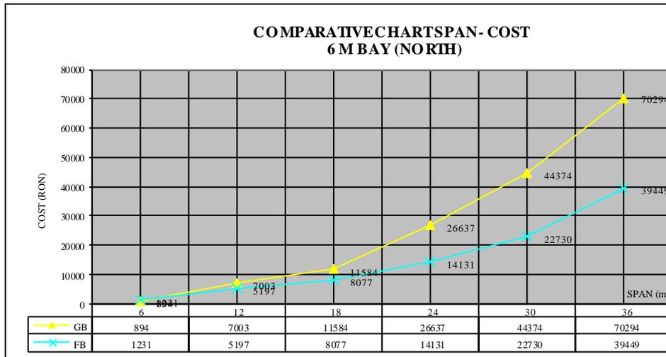
Fig. 4. Comparative chart span - cost. 6 m bay
