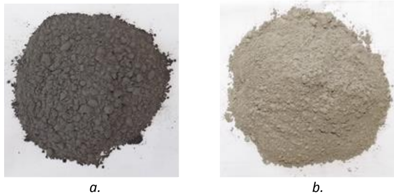
Fig. 1. The aspect of corn cob ash (a), comparatively presented to cement (b)
