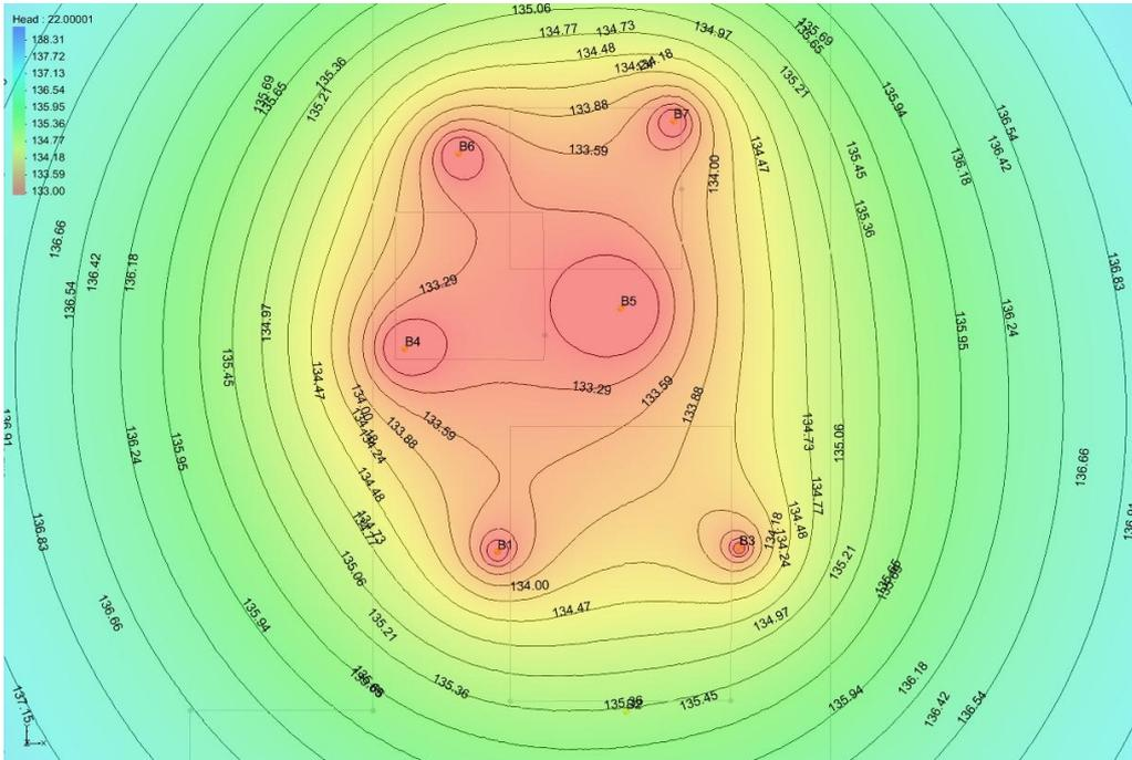
Fig. 7. Groundwater levels after 22 days (operative wells B1, B3, B4, B5, B6 and B7)
