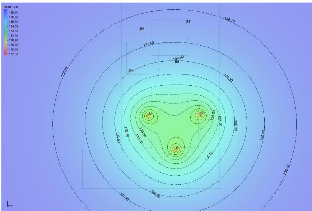
Fig. 5. Groundwater levels after 4 days (operative wells B1, B2 and B3)
