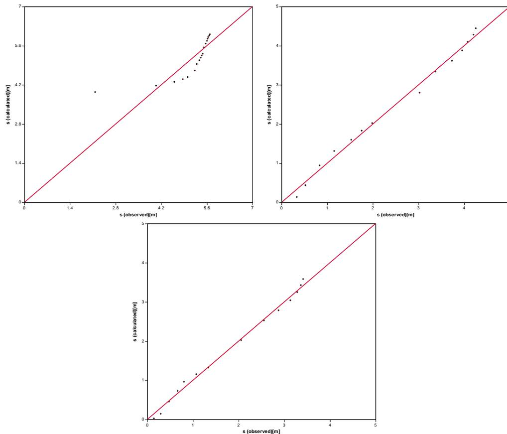
Fig. 4. *Observed vs. calculated drawdown in well and two piezometers*
