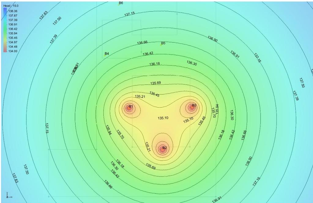
Fig. 6. Groundwater levels after 15 days (operative wells B1, B2 and B3)
