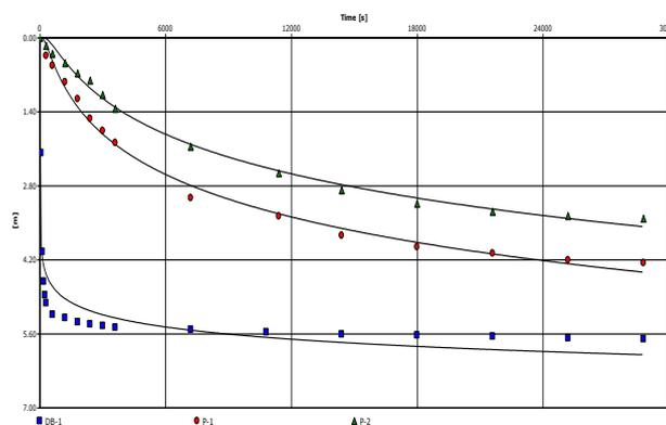
Fig. 3. Graphical representation of a pumping test result
