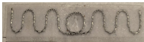
Fig. 7. UHF antenna pattern sewn with conductive textile yarn
