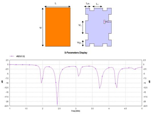
Fig. 1. The initial generator model for fractal patch antenna creation (a)  $0^{th}$  iteration (b)  $1^{st}$  iteration with coaxial feed (c) Simulated loss of return for the  $1^{st}$  Minkowski fractal antenna iteration
