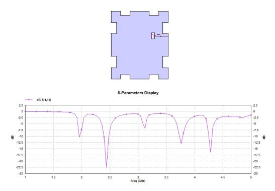
Fig. 2. (a) Antenna structure with optimized dimensions of Minkowski loop; (b) Simulated return loss for modified structure of Minkowski fractal antenna
