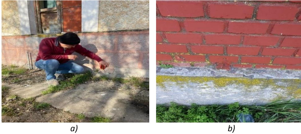
Fig. 2. Bretea point a) static measurements. From the station there is direct visibility to the leveling benchmark embedded in the wall of the building; b) the leveling benchmark
