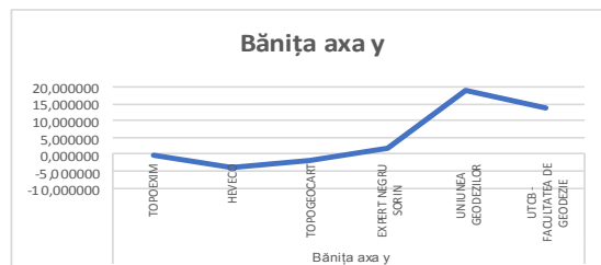
Fig. 8. Differences for the coordinate y between the ROMPOS and static determinations for the Băniţa point
