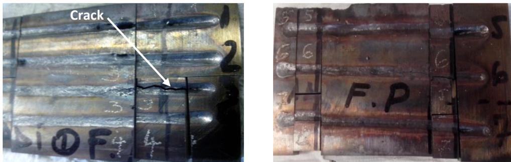
Fig. 1. Fusion lines obtained on ADI with laser beam welding without preheating
