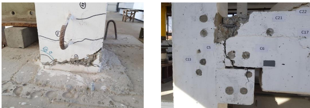
Fig. 7. Degradations of the Model Frame after first experimental test (without lateral stiffeners)
