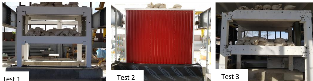
Fig. 6. Test 1: Non stiffened; Test 2: Two-sided stiffened; Test 3: Removal of the corrugated sheets stiffening effect
